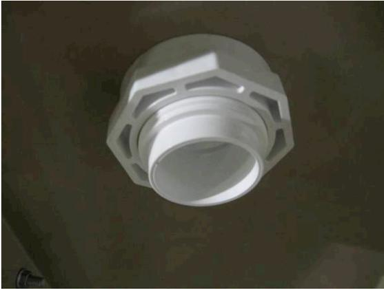
To install the return fitting, you need to un-thread the retaining nut from the fitting. Insert the threads through the pre-punched hole from the inside of the pool and tighten the retaining nut to the back of the fitting. Do not over tighten this nut.
