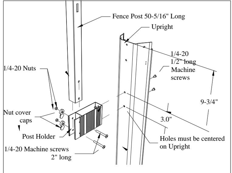
If you are installing a deck on your pool, then part of the deck support system must be installed on your pool uprights **BEFORE** you install the uprights on the pool.
