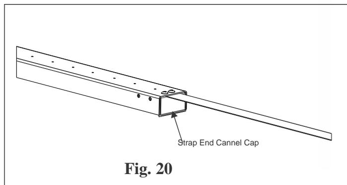
**ALTERNATE STEP 6 -ATTACHING STRAPS TO STRAP END CHANNELS FOR A BUTTRESS-FREE OVAL POOL ONLY:**
