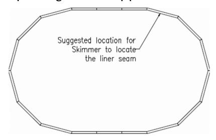
There are several steps that need to be followed before placing the panels into position. Each panel must be marked on the inside face with a line 1½"up from the bottom. This line will mark the finished level for the pool bottom under the liner. The next step is to install the top seat.
