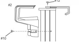
1) Attach the inner top cap using a #12 Screw into hole #2.
