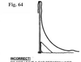
DO NOT LEAVE A GAP BETWEEN LINER AND COVE. THIS WILL CAUSE DOWN-WARD PRESSURE ON THE LINER. CORRECT THIS CONDITION IF IT OCCURS.
