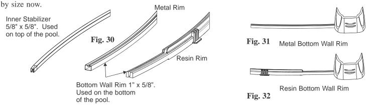
\* IMPORTANT: Make sure you are using the bottom rails and not the inner stabilizer bars. The bottom rails on some pool models are made of resin and not metal (see Fig. 31 and Fig. 32). The stabilizer bars are always metal and they have male and female end. The bottom rails are the larger width rails that have the straight cuts on both ends. The bottom rails do not interlock (see Fig. 30).
