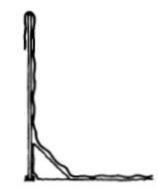
CORRECT NO AIR SPACE BETWEEN LINER AND POOL - SLACK ON SIDES.
