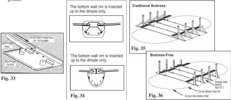
IMPORTANT: Some pools have resin bottom plates or resin bottom cuffs rather than the traditional metal bottom plate. Please refer to yourpool parts breakdown sheet to confirm which component applies to you particular pool.
