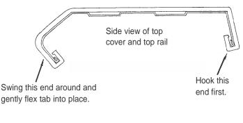
Bullnose rail is used for the illustration, but installation is the same for all 1 pc. clip-on resin covers.
