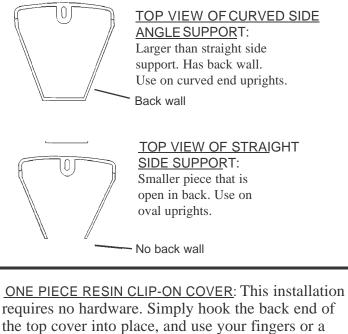
the top cover into place, and use your fingers or a screwdriver to gently flex the front tabs enough to hook the cover in place. Make sure that the top cover is centered over the upright when installing.
