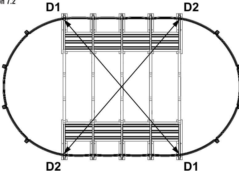
The two measurements, D1 and D2, should be exactly the same. If they are not, adjust one entire straight side as necessary.
