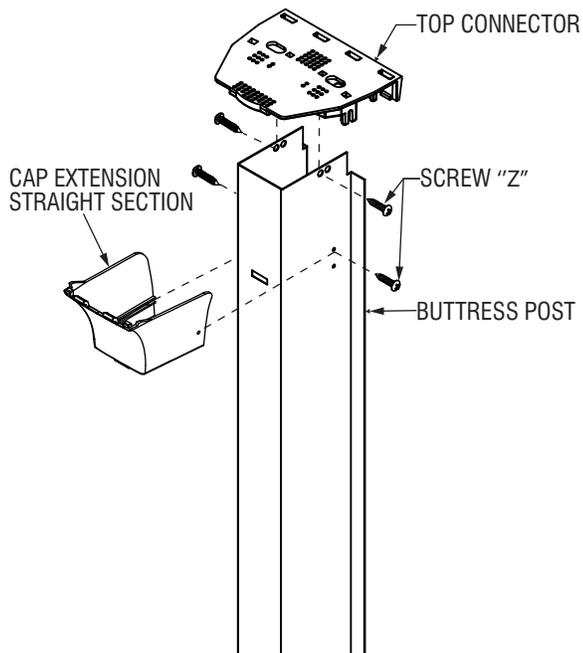
Install the top connector into the uprights and secure with 1 screw "Z" on each side. Install the cap extension into the buttress post with 1 screw "Z" on each side.
