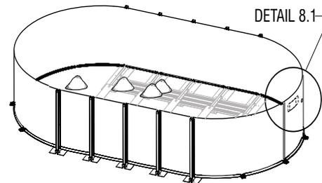
as per chart 1.4 (next page), adjust tracks and bottom connectors and if applicable, uncoil the wall again. If the spread is too wide, measure the wall and check it against the chart of actual wall lengths below. Join both ends of the wall by orienting folds outward to hide the exclamation icon per illustration below.
