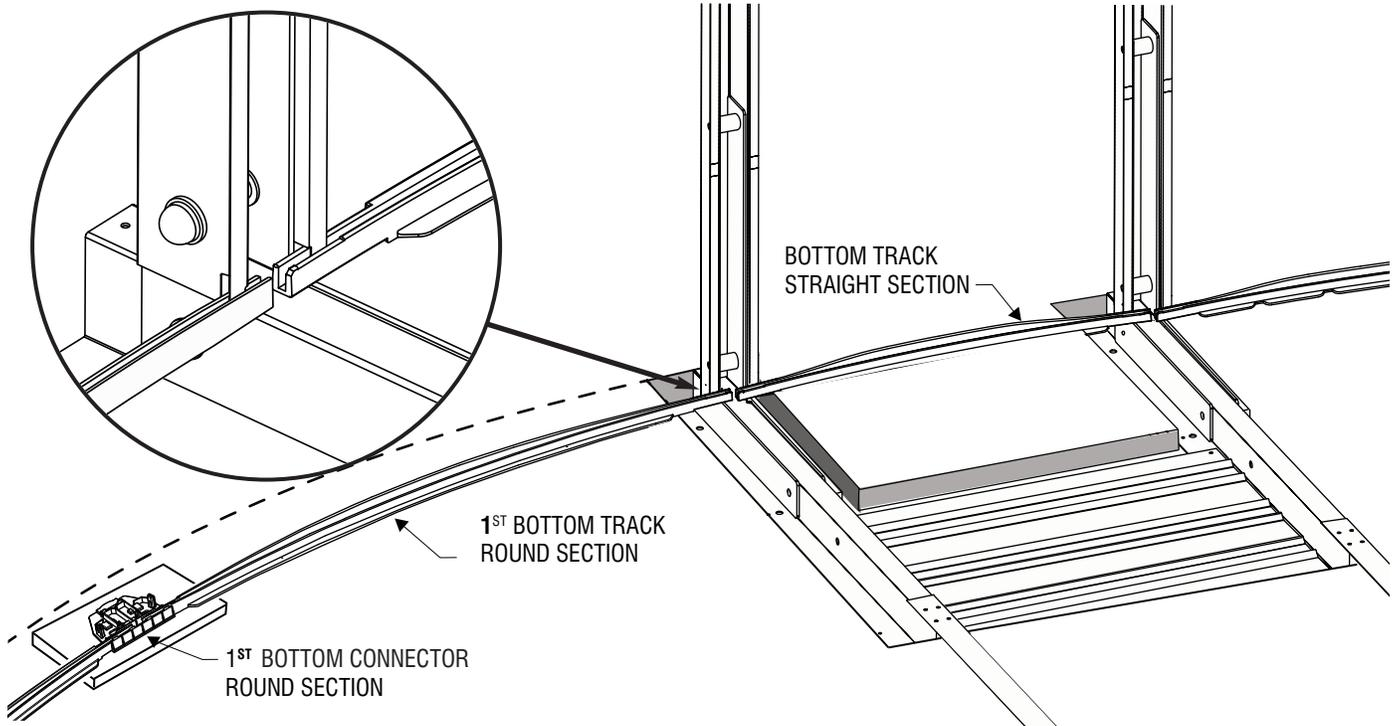
**Important :** Before going to the next step, make sure that the centre of the pool is properly squared and the tension straps are straight with no buckles. Refer to illustration 7.2.
