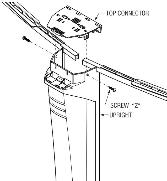
Install the top connector into the upright and secure with 1 screw "Z" on each side.
