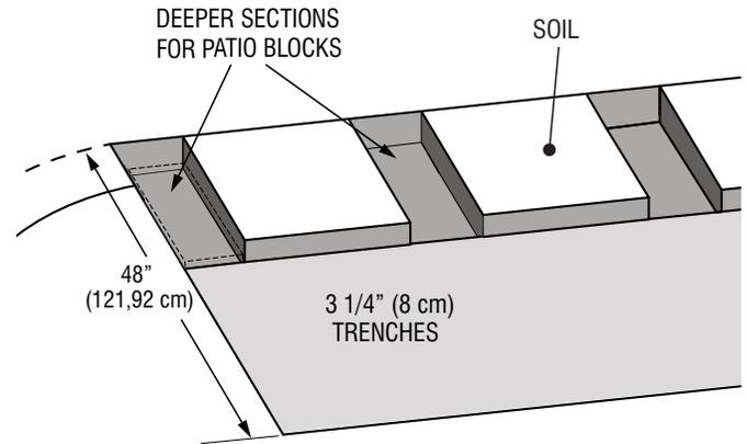
of patio block is 3 1/4" (8 cm) deep in order to accommodate for the buttress assembly thickness. (Refer to illustration 2.4) Top of buttress assembly must be level with the soil.
